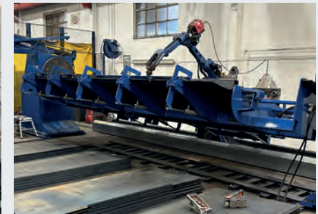
(SAP automated robot welder)
