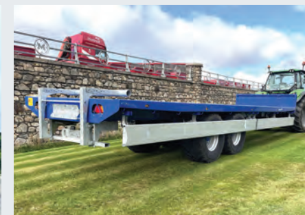
(Rear integrated lights, box pusher and hydraulic side step)
