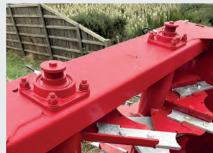
(Rear rotor bearings)
